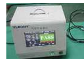
Air leak tester (test sealing of lights)
